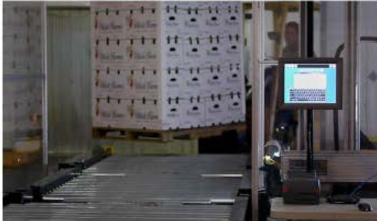
Pallet is placed onto rollers
