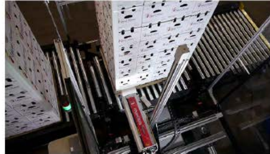
Camera reads the pallet tag as the pallet enters the system
