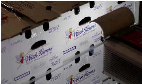
Camera locates the film patch pre-applied by the box manufacturer
