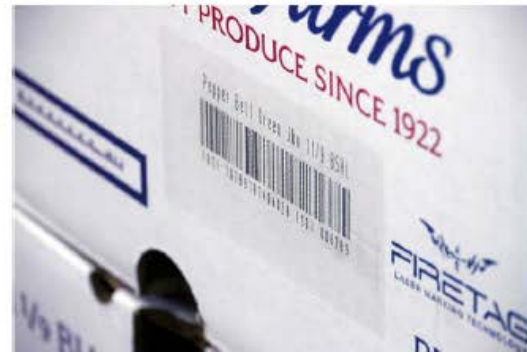
The laser brands each box with specific barcode information
